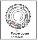
An FA zoom lens without the power supply contacts are shown in the illustration does not have the power zoom function (ie: FA28 - 70mm f / 4 AL lens).
